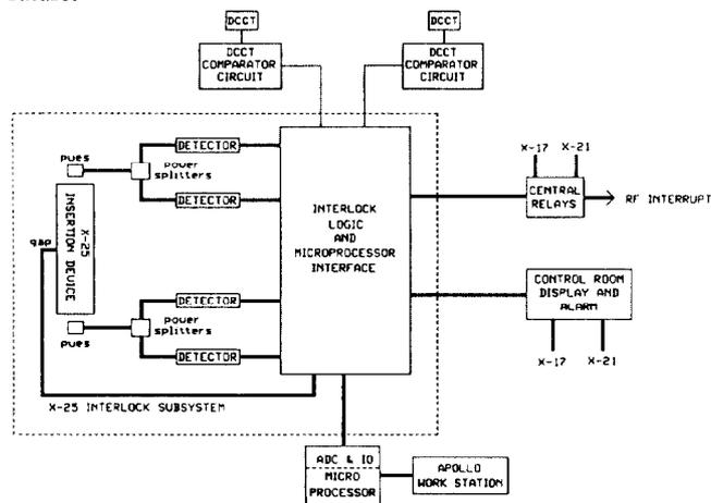
Fig. 3 Active interlock block diagram.
