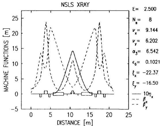
Fig. 4 X-ray ring machine functions.
