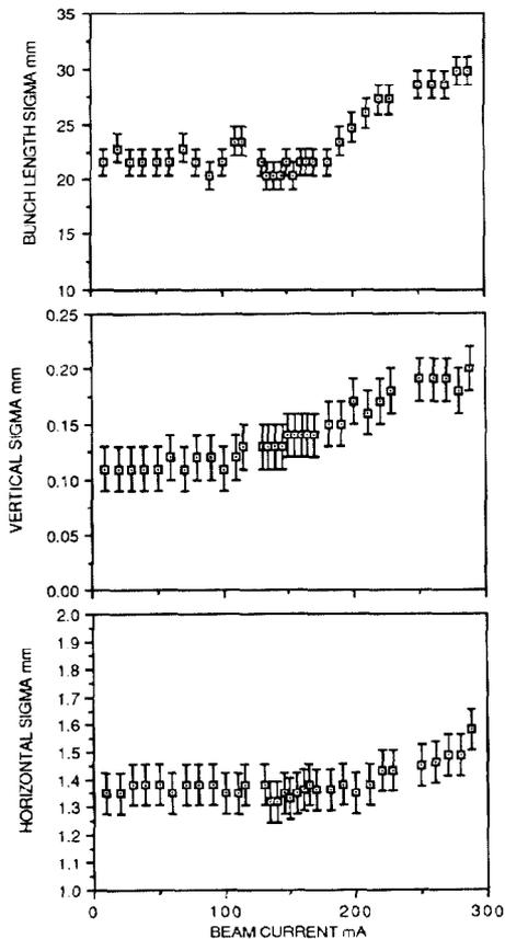
Fig. 3. Beam size variation with beam current.
