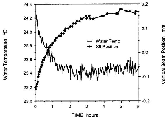
Fig. 6. Correlation between cooling water temperature and radiation beam position.
