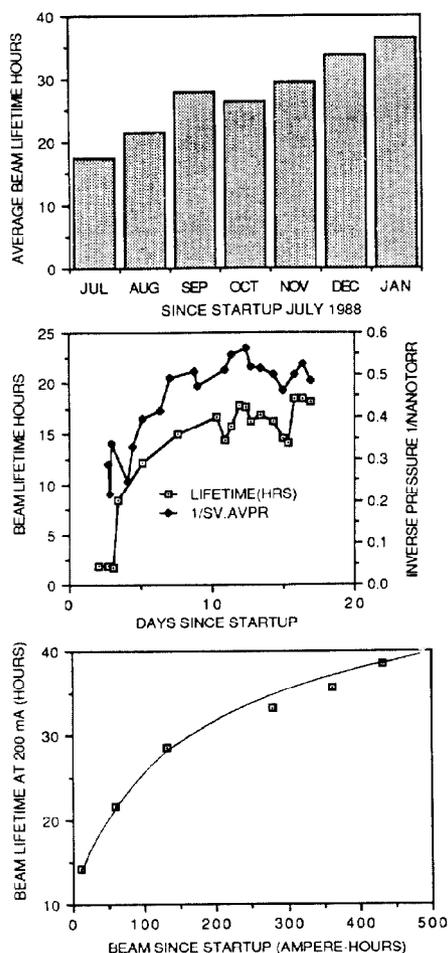
Fig. 5. Improvement in lifetime after a partial vacuum let-up in July 1988.
