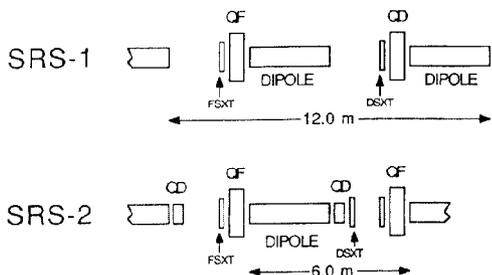
Fig. 1. Comparison between old and new SRS lattices.
