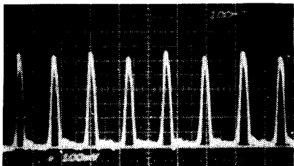
Fig. 8. Eight pulse burst current after magnet traversal.
