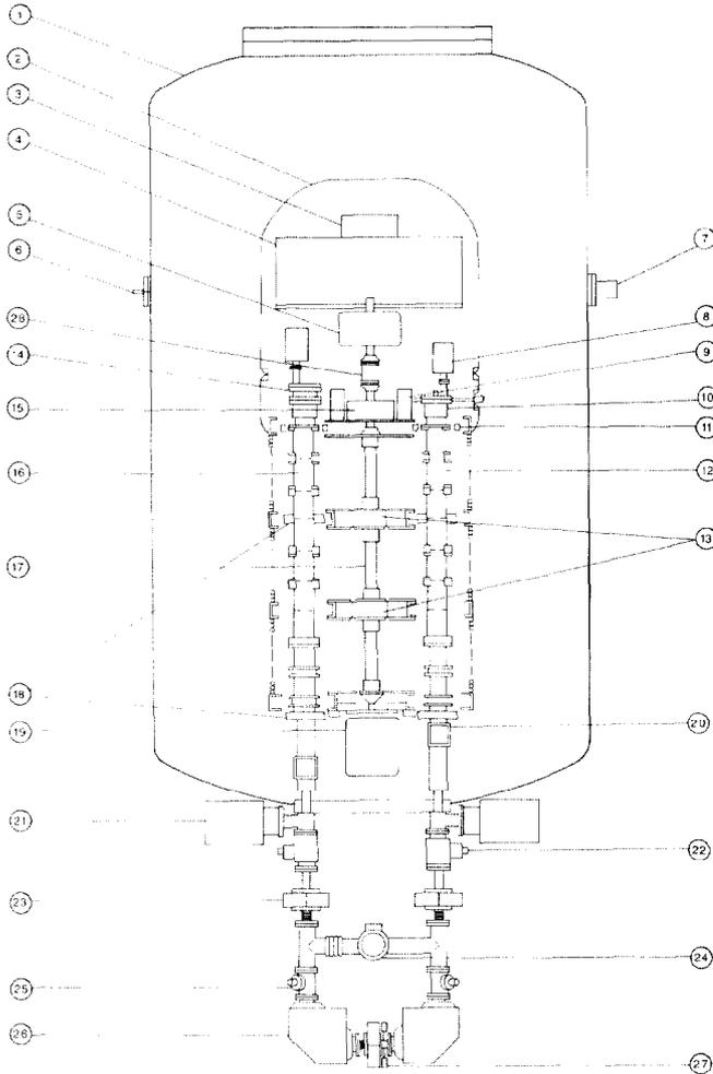
Figure 2: Overall system schematic: 1) tank, 2) high voltage terminal, 4) gun and collector electronics box, 5) 10 kVA generator, 10) gun, 11) steerer coils, 12) acceleration tube, 14) collector, 17) rotating shaft, 18) solenoid lenses -4, 22) Faraday cups -2, 23) quadrupole singlet -3, 25) beam profile monitor -2, 26) dipole -2.
