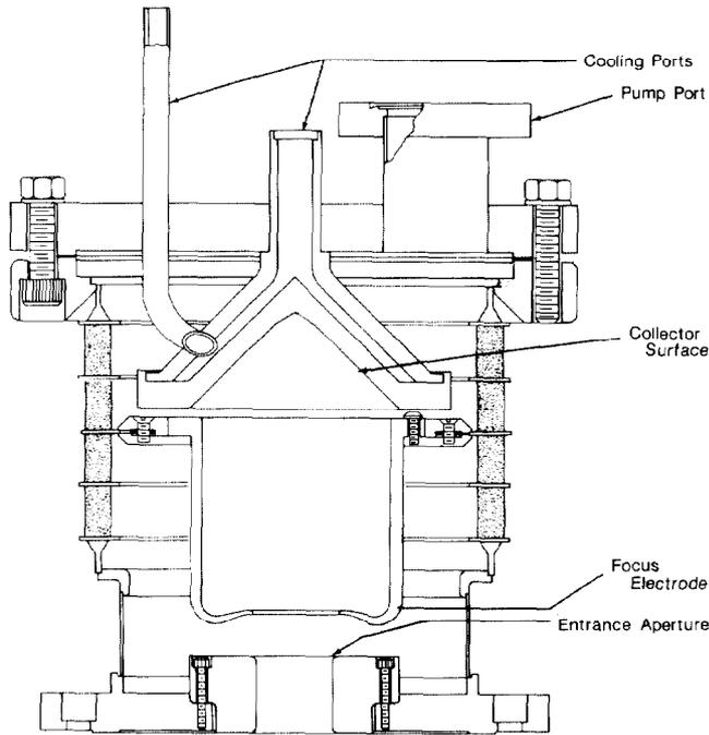
Figure 4: Electrostatic collector: Entrance aperture typically at 33 kV, with respect to gun cathode, focus electrode at 0 kV and collector surface at 5 kV.
