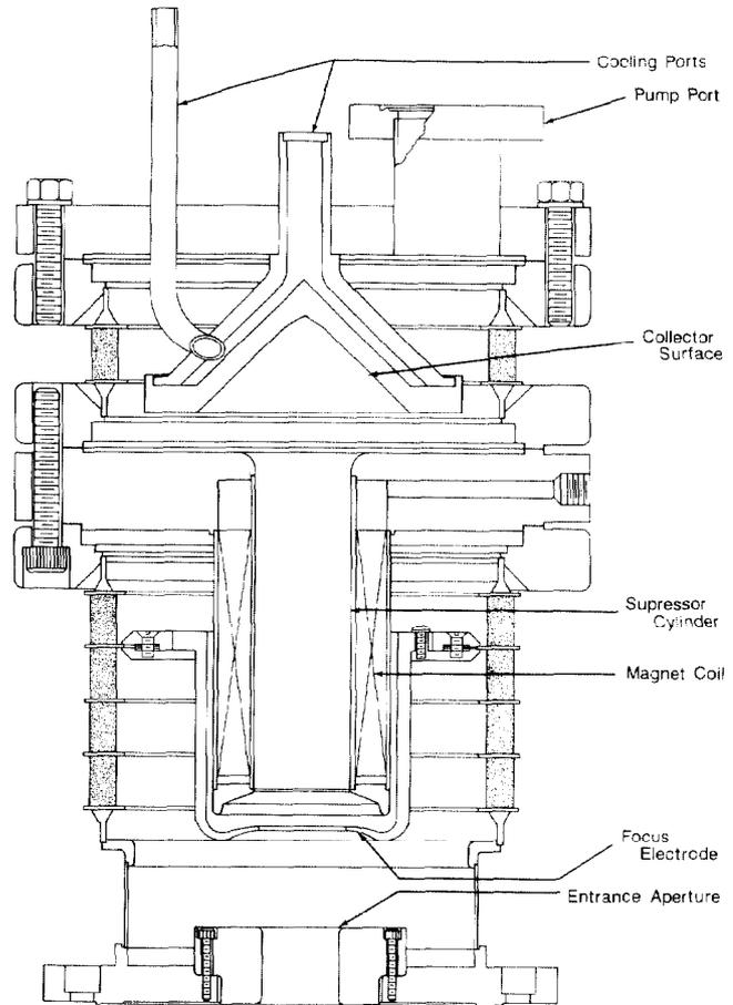
Figure 3: Solenoid/Electrostatic well collector: Entrance aperture typically at 33 kV with respect to gun cathode, focus electrode at 6.5 keV, suppressor at 1.2 kV - 1.4 kV, and collector surface at 5 kV.
