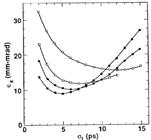
Fig. 2 The emittance as a function of the pulse length and the accelerating field  $E_o$ . The simulation parameters are  $f = 1269$  MHz,  $Q = 2$  nC,  $\sigma_x = 3$  mm, and  $E_o = 40$  (o),  $60$  (□),  $80$  (●) and  $100$  MV/m (■).
