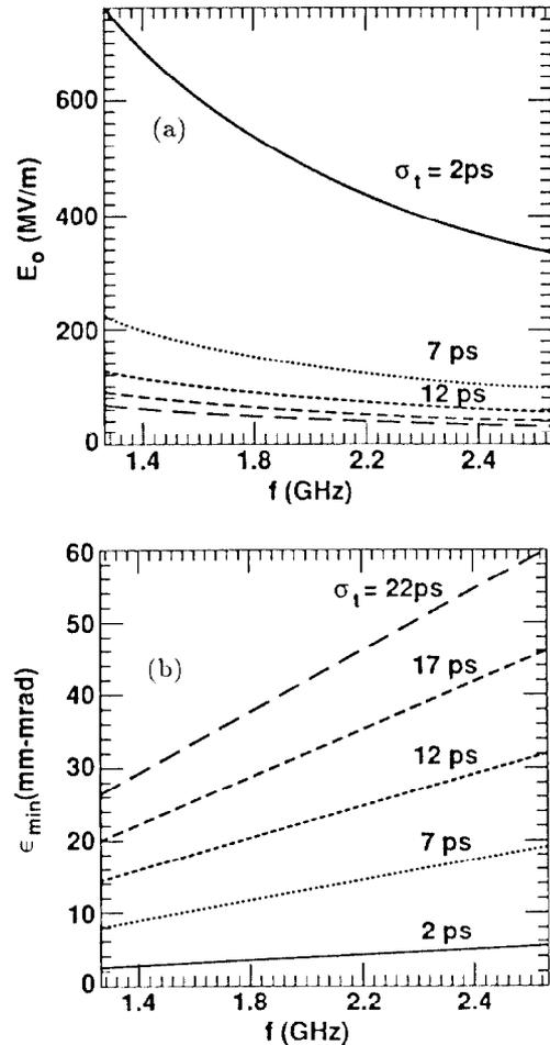
Fig. 3 (a) The optimal accelerating electric field and (b) the minimal normalized emittance for an electron bunch with a peak current  $I = 100$  A and a radius  $\sigma_x = 3$  mm as a function of the rf frequency and the bunch length.
