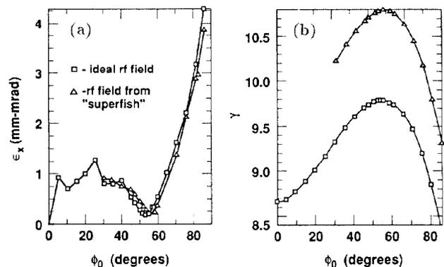
Fig. 4 Comparison of the rf field effects by using a linear rf field ("□") and a rf field calculated by SUPERFISH ("△") for a rf gun described in Table I, Case 1. (a) The emittance  $\epsilon_x^{rf}$  and (b) the dimensionless electron energy  $\gamma$  versus the emitting rf phase  $\phi_0$  are plotted.
