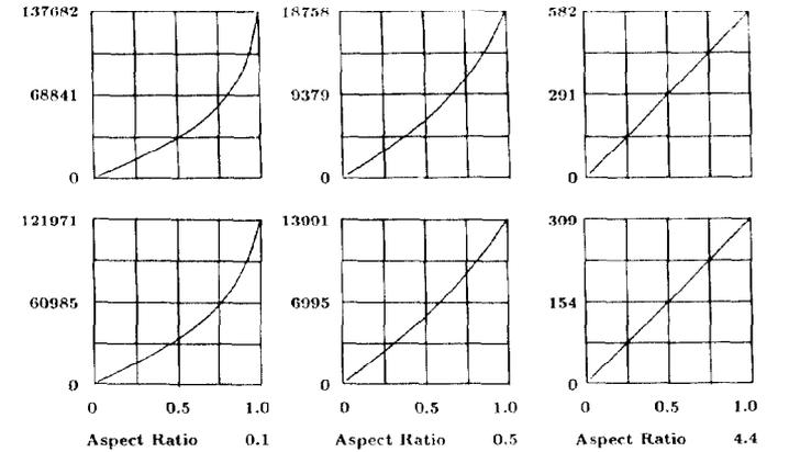
Fig. 2. Radial electric field versus  $\rho$  plots for the axial center (top) and edge (bottom) of the slug beam for some different aspect ratios.
