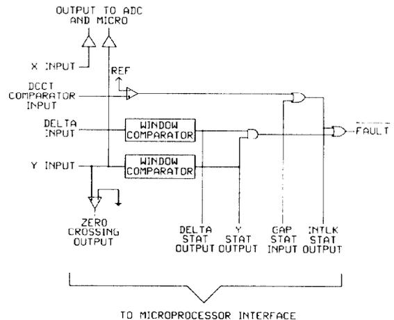
Figure 3. Interlock logic.
