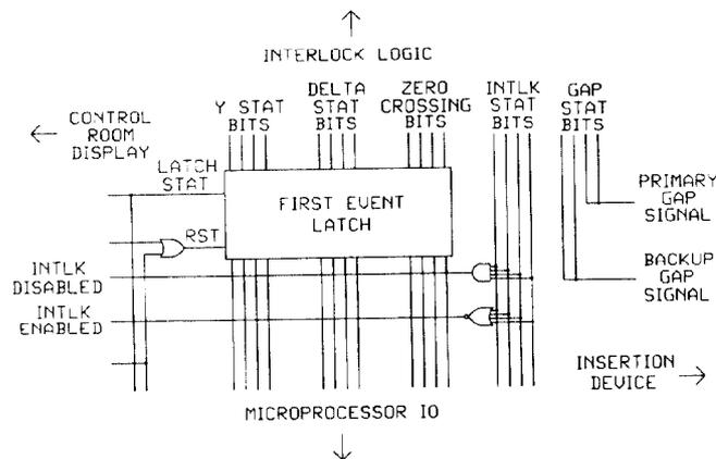
Figure 4. Microprocessor interface.
