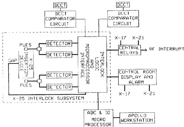
Figure 1. Interlock block diagram.
