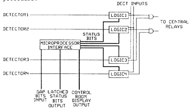
Figure 2. Interlock logic & microprocessor interface.
