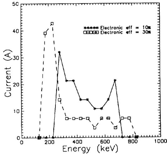
Figure 2. Energy spectrum of spent beam from 30 MW gyrokylystron. The initial energy is 500 keV, the current, 150 A. Spectra for electronic efficiencies of 10% and 30% are given.
