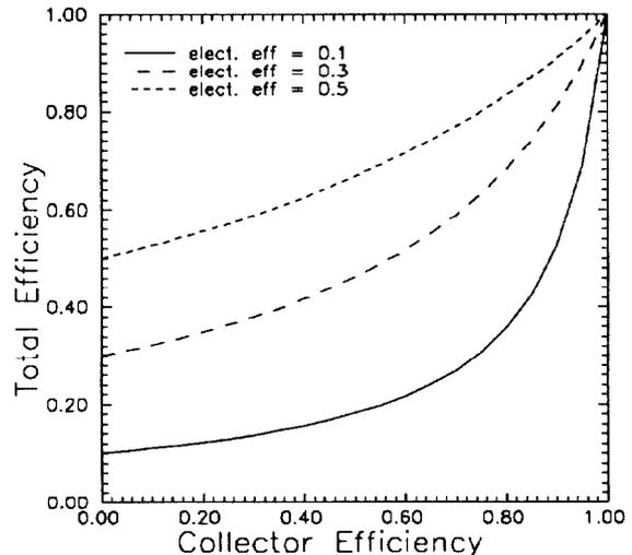
Figure 1. Total efficiency of a microwave tube with a depressed collector, as a function of the collector and electronic efficiencies.
