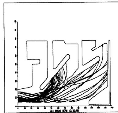
Figure 4. Trajectories of the primary electrons for the collector of Figure 3.
