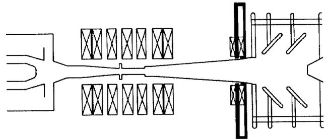
Figure 3. Schematic of a depressed collector for a 10 GHz, 30 MW gyrokylystron, with a beam energy of 500 keV and a current of 150 A.
