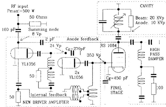
Fig. 2. Schematic of the cavity amplifier plug-in.
