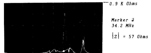
Fig. 6. Anode impedance with/without damping circuit (10 - 50 MHz).
