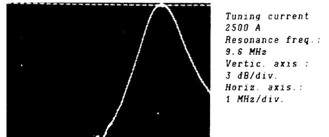
Fig. 5. "Typical" closed loop transfer functions.
