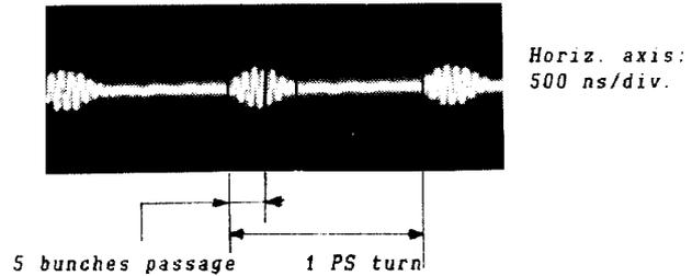
Fig. 9. Transient beam loading.
