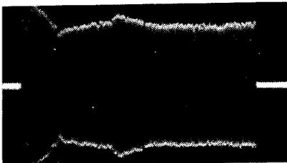
Fig. 7. Beam induced voltage without RF feedback.
