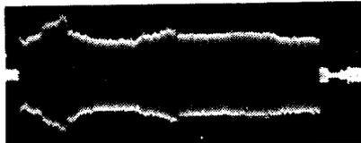
Fig. 8. Beam induced voltage with RF feedback.
