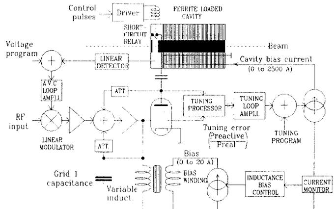
Fig. 4. Cavity and amplifier servo systems
