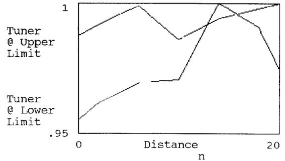
H Field Distribution vs. Tuner Loop Position
