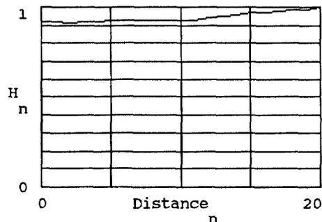
*Measured H Field Distribution In Cavity 3*
