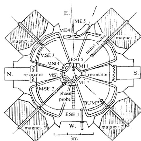
Fig.4: The schematic diagram of the main accelerator SSC.
