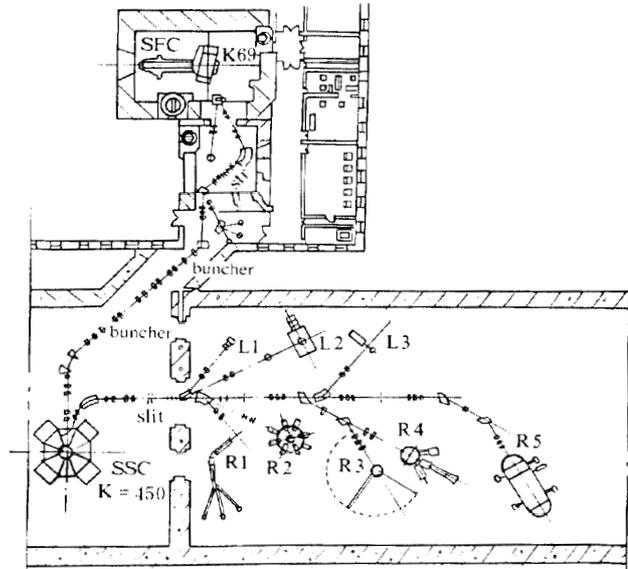
Fig.1: General layout of HIRFL. R1-isotope separator, R2-in beam  $\gamma$ -measuring devices, R3-heavy ion telescope, R4-position sensitive ionization chamber, R5-cylindrical scattering chamber, L1-fast chemical separation apparatus, L2-irradiation equipment, L3-equipment for atomic physics study.
