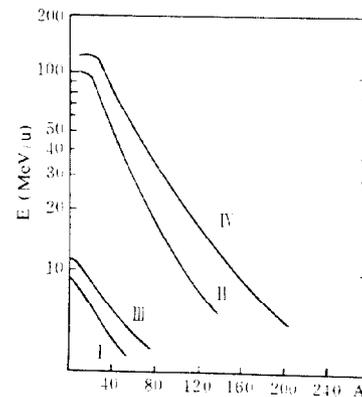
Fig.2: The maximum energy vs. mass number of HIRFL.
