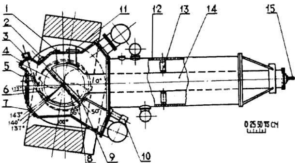
Fig.3: Schematic diagram of the injector SFC. 1-measure capacity, 2-probe, 3-steering magnet, 4-ion source, 5-magnetic channel, 6-deflection plate, 7-probe, 8-dummy dee, 9-dee, 10-coupler capacity, 11-trimmer capacity, 12-cavity, 13-shouted plate, 14-dee stem, 15-probe.
