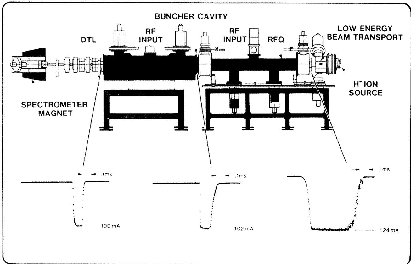
Figure 1. The Accelerator Test Stand at Los Alamos National Laboratory (LANL). The current traces indicate both the bunching of the ion source beam in the RFQ and the high transport efficiency through the RFQ and DTL.
