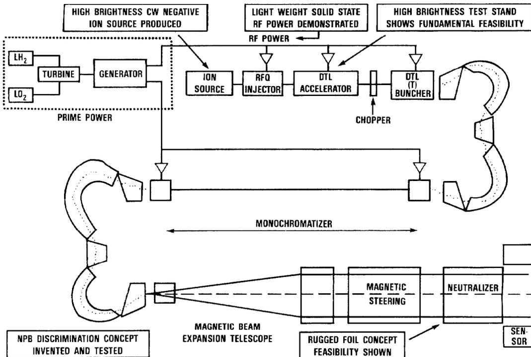
Figure 2. This NPB block diagram shows significant progress in RF power, ion sources, emittance preservation, and foil neutralizers.
