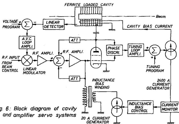
Fig. 6: Block diagram of cavity and amplifier servo systems
