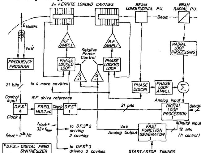
Fig. 2: Simplified block diagram of low level R.F.
