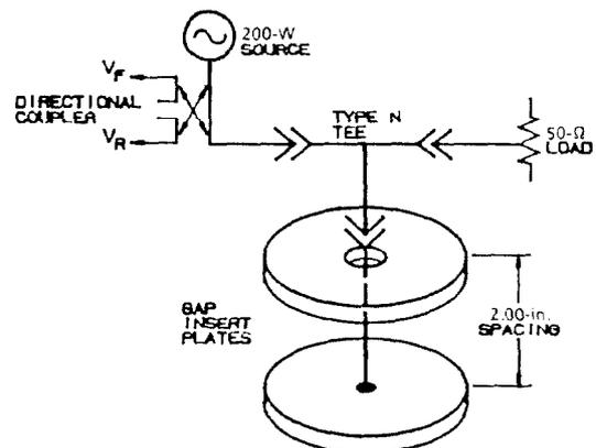
Fig. 2. Gap voltage calibration circuit.
