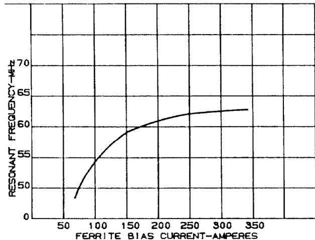
Fig. 3. Cavity tuning curve.
