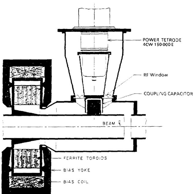
Fig. 1. Cross section of cavity amplifier.
