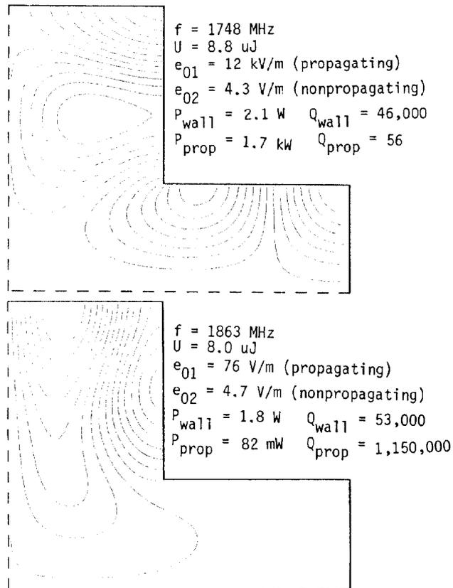
FIGURE 5: UNTRAPPED AND TRAPPED CAVITY MODES. AMPLITUDES OF WAVEGUIDE MODES, PROPAGATING POWER AND Q<sub>s</sub> ARE SHOWN
