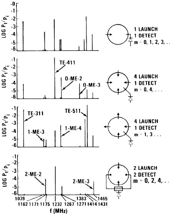
FIGURE 1: SELECTIVITY IS USED IN ISOLATING AND IDENTIFYING MODES
