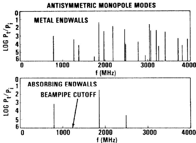
FIGURE 4: ANTISYMMETRIC MONOPOLE MODES, WITH CONDUCTING ENDWALLS AND ABSORBING ENDWALLS
