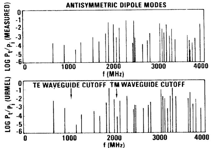
FIGURE 3: ANTISYMMETRIC DIPOLE MODES, MEASURED AND CALCULATED
