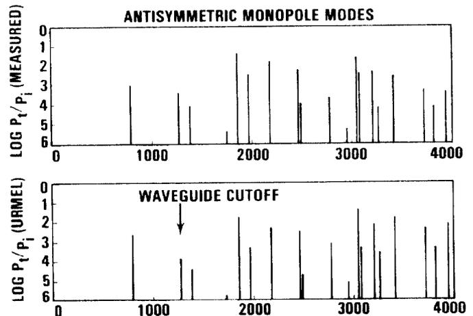
FIGURE 2: ANTISYMMETRIC MONOPOLE MODES, MEASURED AND CALCULATED
