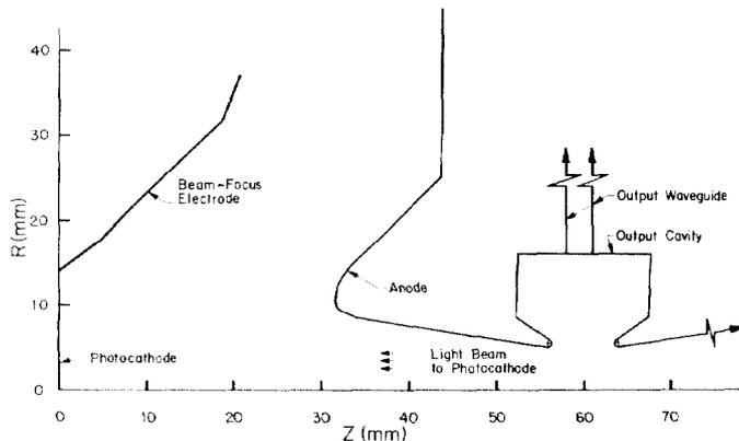
Fig. 1. Schematic diagram of the 6-GHz Orsay prototype lasertron.
