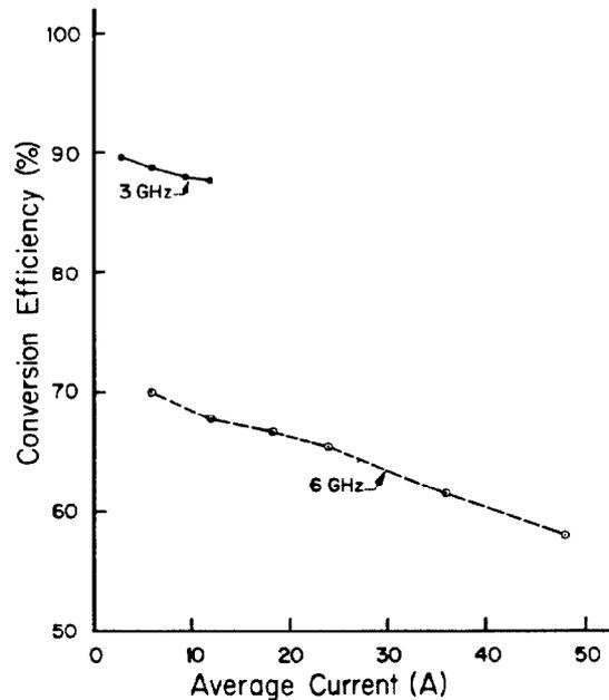
Fig. 3. Calculated dc to rf conversion efficiency versus peak beam current for the Orsay prototype lasertron at 3 and 6 GHz and 300 kV.
