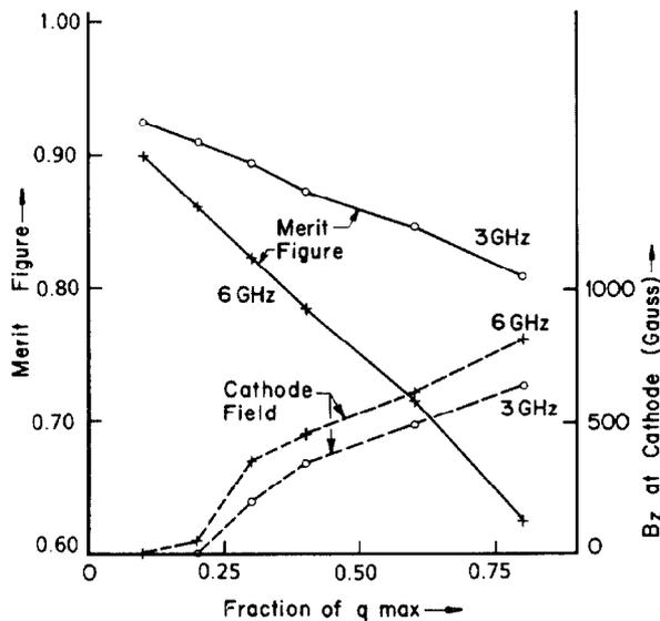
Fig. 2. Merit-figure estimate of efficiency and magnetic-focus field versus fraction extracted of  $q_{max}$ : planar acceleration fields, Bessel function space-charge fields,  $r_c = 15$  mm, frequency = 3 and 6 GHz,  $V_0 = 300$  kV, anode-cathode distance = 30 mm.
