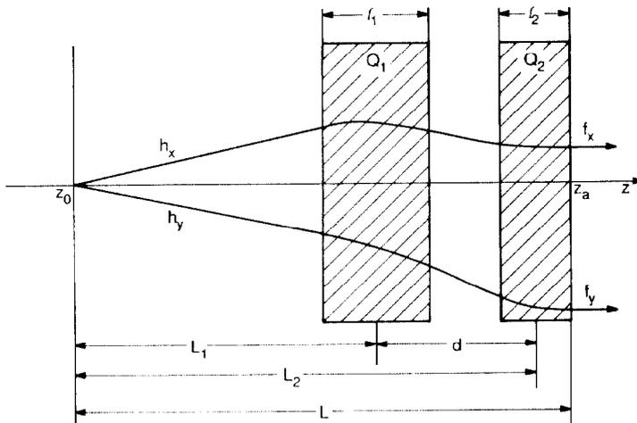
Fig. 1. Schematic description of a quadrupole doublet.
