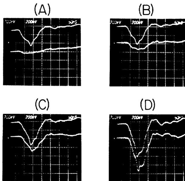
Fig. 3. Rogowski signals for beam transport in hydrogen gas. The upper trace is from Rogowski 1 (0.5 kA/div) and the lower trace is from Rogowski 2 (0.6 kA/div). 50 ns/div.
