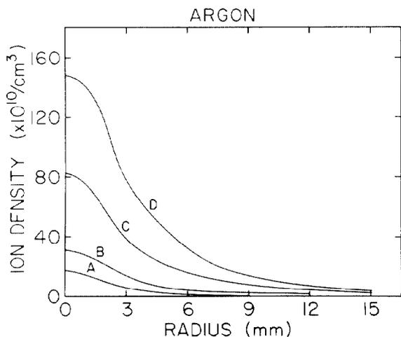
Fig. 2. Ion density profiles for argon gas.
