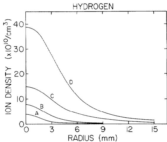
Fig. 1. Ion density profiles for hydrogen gas.
