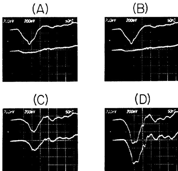
Fig. 4. Rogowski signals for beam transport in argon gas. The upper trace is from Rogowski 1 (0.5 kA/div) and the lower trace is from Rogowski 2 (0.6 kA/div). 50 ns/div.
