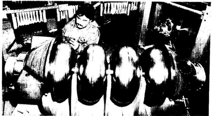
Fig. 3 4-cell Nb-cavity before closing the LHe container.
