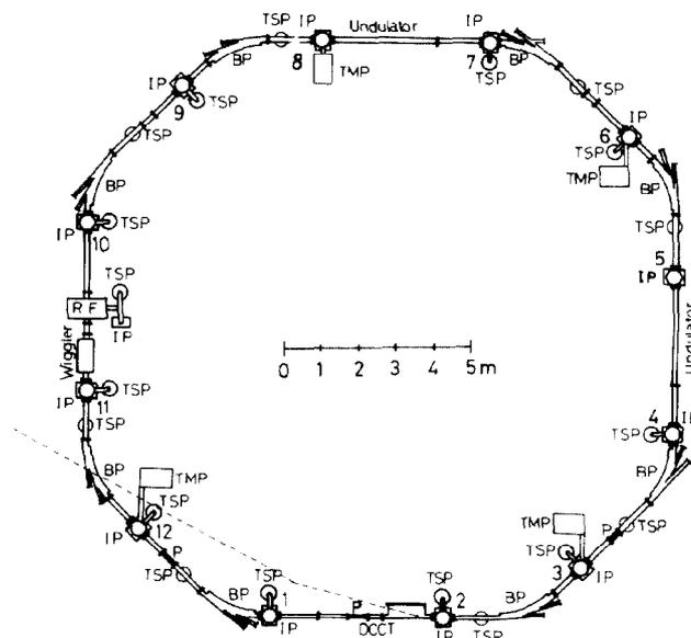
Fig. 1. Plane view of vacuum doughnut of UVSOR. IP: sputter ion pump, TSP: titanium sublimation pump, BP: built-in pump, TMP: turbo-molecular pump, P: perturbator chamber, DCCT: DCCT chamber, I: inflector chamber and 1-12: vacuum gauge.
