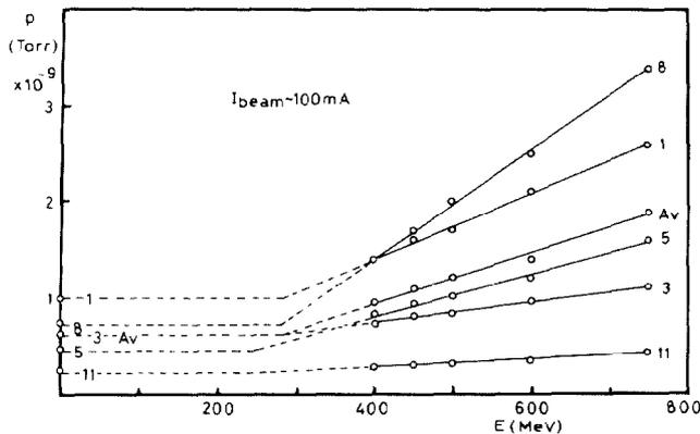
Fig. 4. Dependence of pressure on electron energy.
