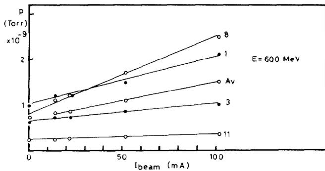
Fig. 3. Dependence of pressure on beam current.
