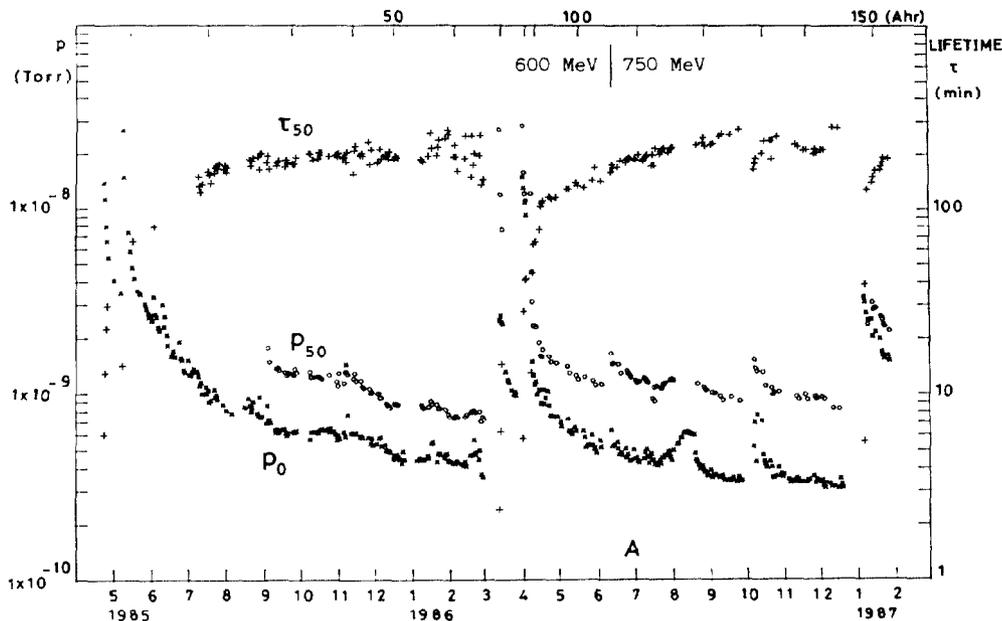
Fig. 2 Improvements of pressure and lifetime.  $P_0$ : base pressure,  $P_{50}$ : pressure at 50 mA and  $\tau_{50}$ : lifetime at 50 mA. Horizontal axis shows date and integrated beam current (Ahr).
