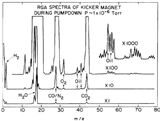
Fig. 2. The RGA spectra of the FEB kicker magnet during pumpdown.
