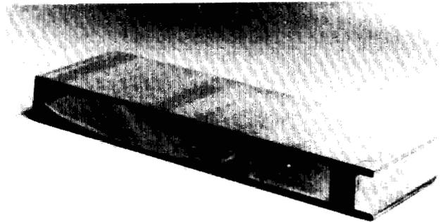
Fig. 2. Photograph of the aluminum-extruded vacuum chamber.
