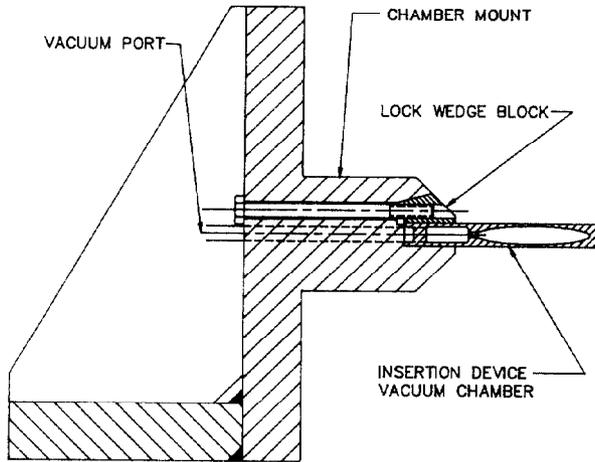
Fig. 3. Cross-sectional view of the vacuum chamber mounted in the chamber mount structure. The vacuum port slots and tightening screw rods are located at different places along the longitudinal direction of the chamber.
