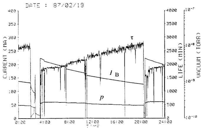
Fig.4 Pressure, beam life time and the beam current on February 2 in 1987. Injected beam current was 225 mA, and average pressure of the ring was less than  $3 \cdot 10^{-10}$  Torr. Beam life time was over 1700 minutes at 220 mA of the beam current, and reached 2700 minutes just before the next injection.
