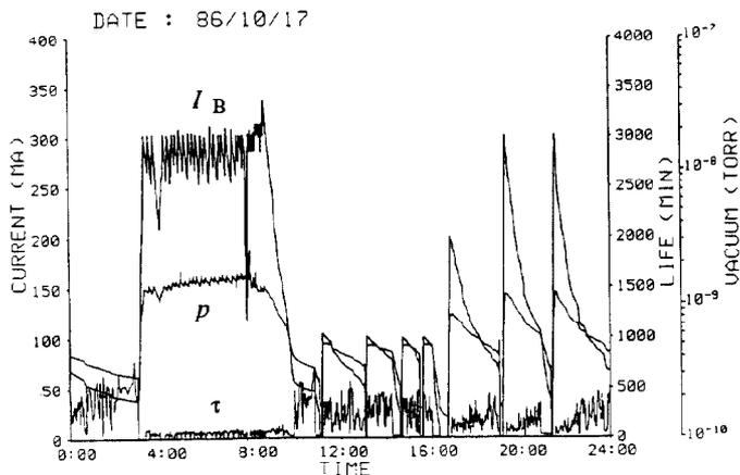
Fig.3 Pressure change on October 10 in 1986 after the accident of polyethylene rushing. Beam current  $I_B$  and beam life time  $t$  are also shown. The beam was injected frequently at 300 mA in order to clean the vacuum ducts by photons.
