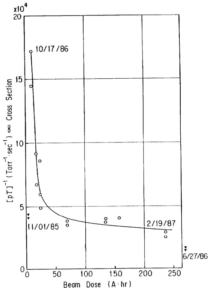
Fig.5 Colliding cross sections with the residual gas molecules. They were expressed as  $1/(p \tau)$  and plotted the beam dose. Open circles indicate the values after the polyethylene accident in the second shutdown, and filled triangles indicate values after the first shutdown. The short beam life time shown in Fig.3 does not caused by the effect of the air exposure during the shutdown but by the contamination by polyethylene rushing.
