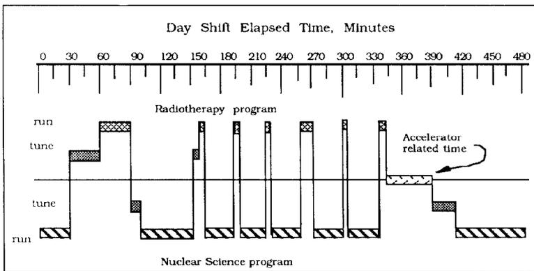
Figure 5. Typical beam sharing during weekday operation of the Bevalac. In this case, radiotherapy dosimetry and 6 treatments are shown interspersed with nuclear science operation.
