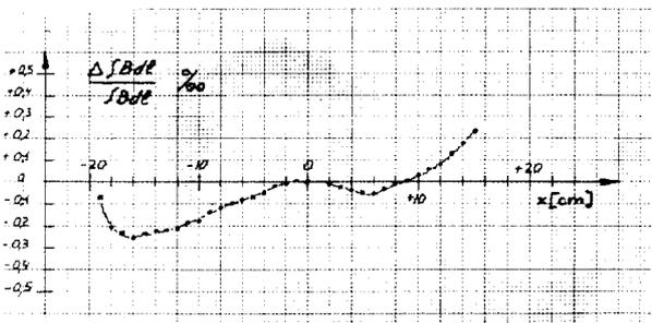
Figure 4c - BHW. Influence of proximity of lattice quadrupoles
