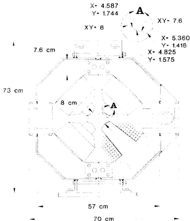
Fig. 2. End View of Quadrupoles
