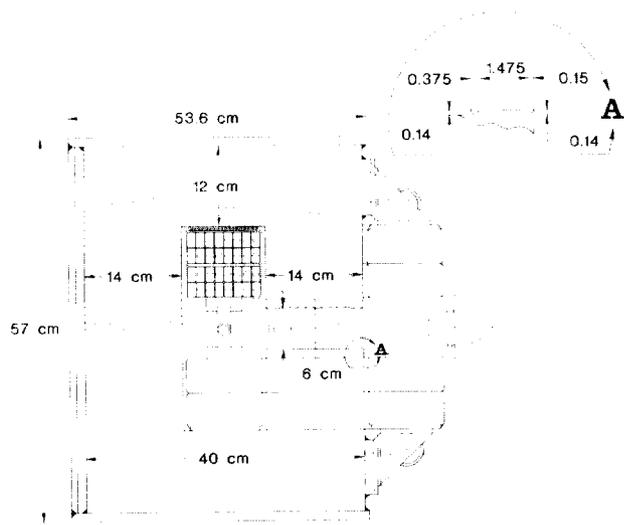
Fig. 1. End View of Dipole
