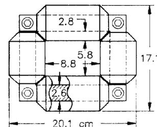
Fig. 5. Vertical/Horizontal Correction Magnet
