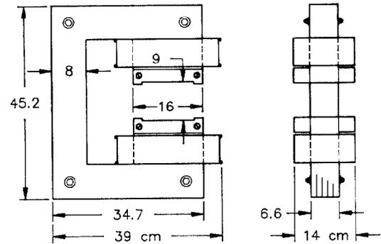
Fig. 4. Vertical Correction Magnet
