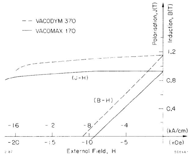
Fig. 3: Demagnetization quadrants of the hysteresis curves for both kinds of rare earth permanent magnets studied. The upper curves give the polarization  $J=B-H$  and the lower ones give  $B$ .
