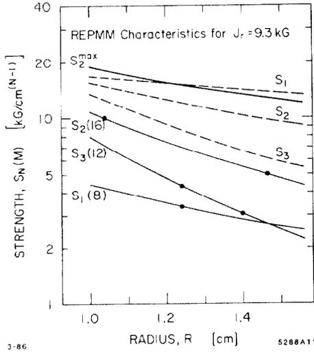
Fig. 2: Strengths of multipoles shown in Fig. 1 for SmCo<sub>5</sub> blocks with  $J_r = 9.3\text{kG}$ . The 8-block quad in Fig. 1 has strength  $2S_2(8) = S_2(16)$ . The dots represent magnets that have been made for the SLC damping rings, their injection and extraction lines and the final focus as shown in Fig. 2.
