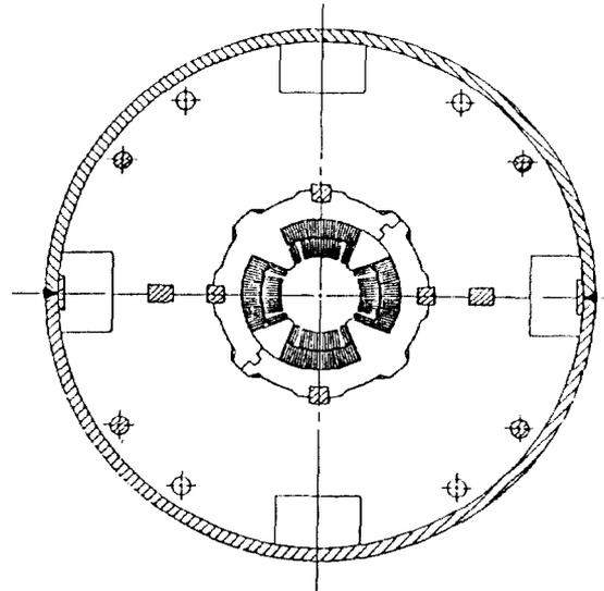
Fig. 4. Cross section of coil in iron yoke.
