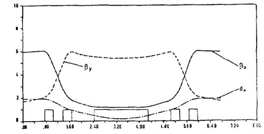
Fig. 8: Twiss functions of Lattice B
