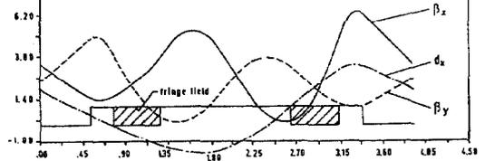
Fig. 7: Twiss functions of Lattice A
