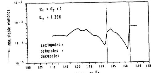
Fig. 9: Horizontal tune vs. maximal stable emittance of Lattice A
