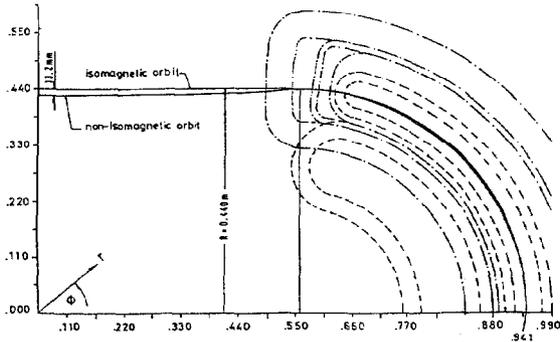
Fig. 1: Top view on the coils arrangement with the isomagnetic and non-isomagnetic orbit.
