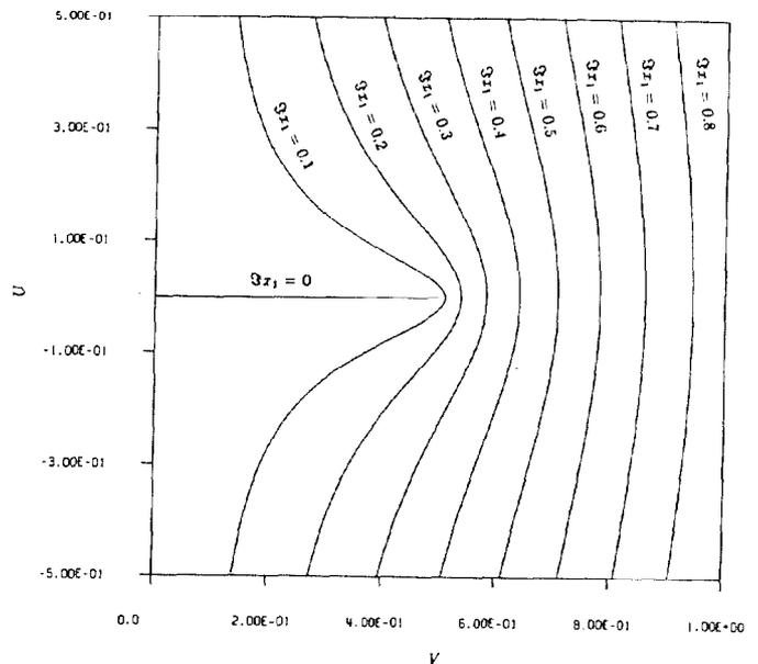
Fig. 1 The stability diagram for the sinusoidal tune modulation
