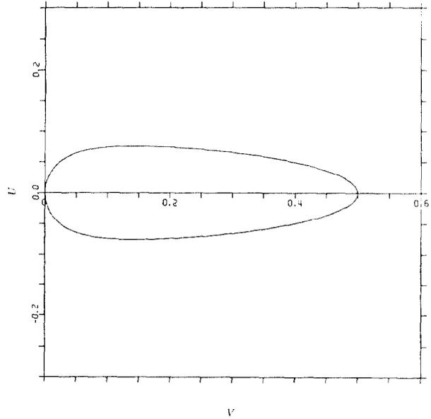
Fig. 2 The stability diagram for the fractionally filled beam. The gap parameter is  $\Delta = \pi/6$ .
