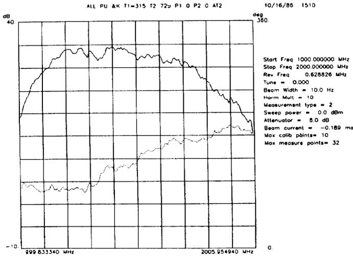
Figure 4. Stacktail Momentum Transfer Function
