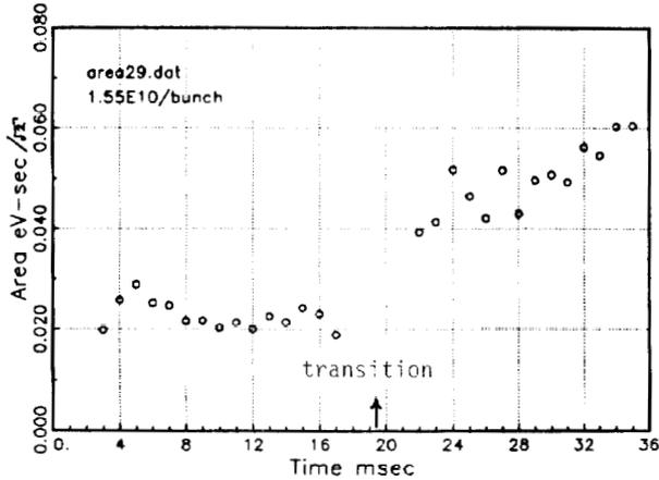
Figure 1: Longitudinal booster bunch area.
