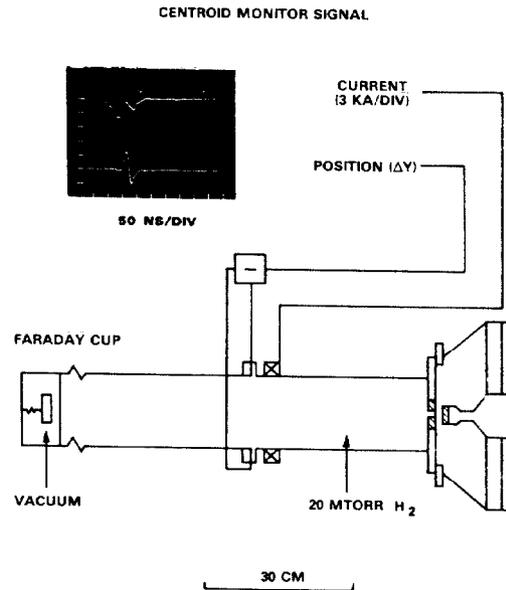
Fig. 2. Beam induced channel experiment showing the location of diagnostics and a 20 mTorr H<sub>2</sub> result.
