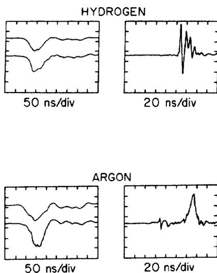
Fig. 3. Pre-formed channel experimental results. The current traces on the left are 1.35 (upstream) and 1.60 (downstream) kAmps/div. The displacement trace is on the right. The calibration for small displacements is 15/I(kA) cm/div.
