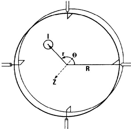
Figure 1. Current centroid displacement probe geometry.
