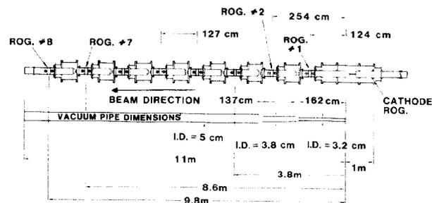
Figure 3. The RADLAC-II beam line.
