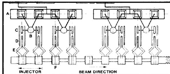
Figure 2. Top view of RADLAC II: (A) intermediate store capacitor, (B) laser-triggered gas switch, (C) pulse forming line, (D) transmission line, (E) convolute, and (F) accelerating cavity.
