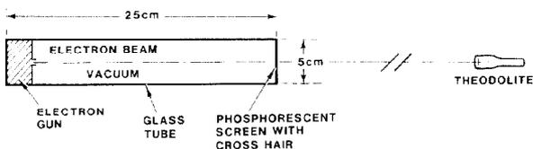
Figure 8. Magnetic alignment electron gun tube.
