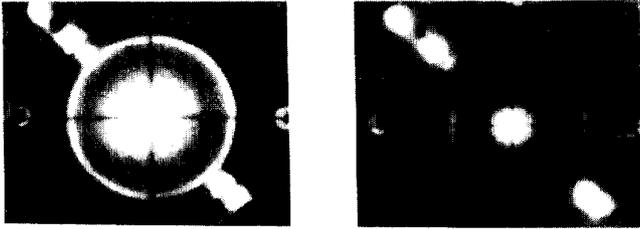
Figure 5. Photograph of the lucite targets inside the accelerator beam line during the alignment process. In the right frame, the target is at the foilless diode anode pipe. In the left frame, the target is located at the exit of the accelerator. In the latter, the target and theodolite cross hair are not rotated relative to each other and completely overlap.
