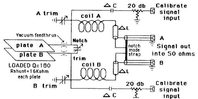
Fig. 4- Schematic of Short Detector
