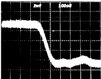
Fig. 3 The pick-up rise-time (inverted) 100 ps/div.
