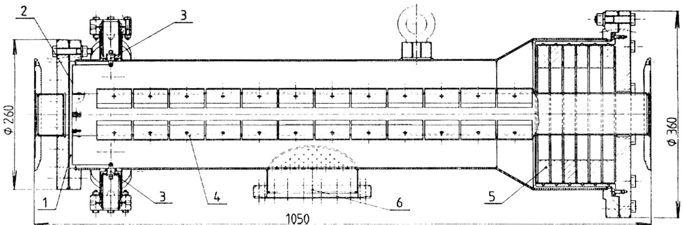
Fig. 1 The wall current monitor: 1, gap; 2, microstrip lines; 3, vacuum feedthroughs (eight) with SMA connectors; 4, absorbing ferrite tiles; 5, ferrite toroids; 6, vacuum-pump connection.
