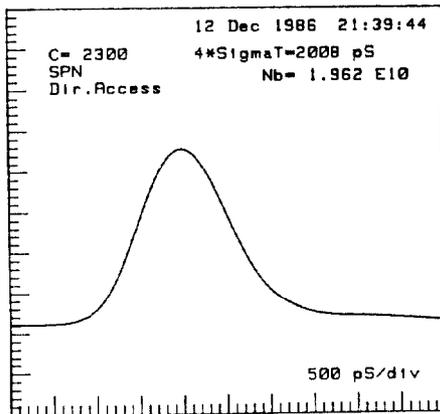
Fig. 8 'Nominal' length electron bunch before extraction
