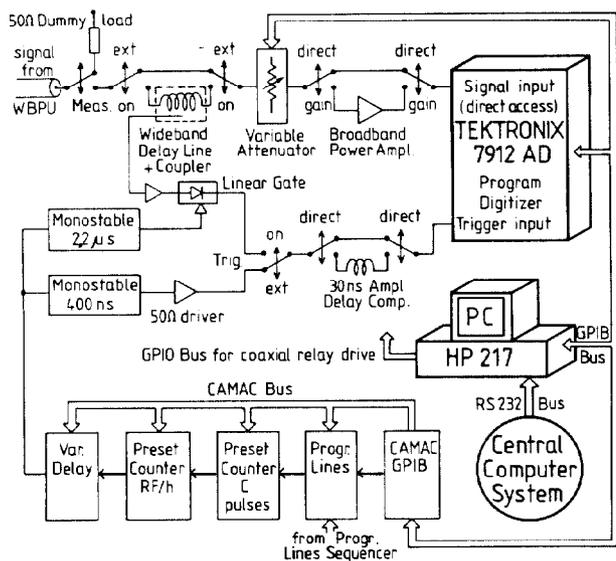
Fig. 4 The data acquisition block diagram
