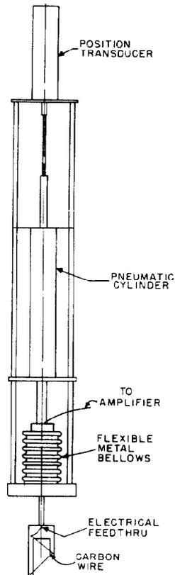
Figure 2. Sketch of a wire scanner.
