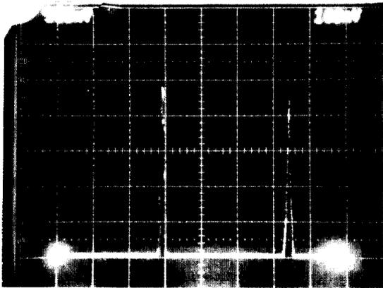
Figure 5. Photograph of wire scanner output to oscilloscope. Horizontal axis is position (3.5 mm/div.), and vertical axis is current. The two peaks correspond to the X and Y beam profiles of a 250  $\mu$ A 5 MeV CW electron beam.
