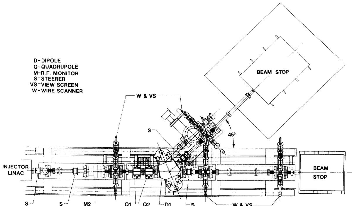
Figure 1. Overhead view of the emittance measuring system for the NBS-LANL RTM 5 MeV injector.
