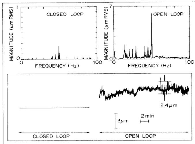
Fig. 3 Beam noise levels taken when the analog feedback loop was either closed or opened. The upper histograms were obtained by using an FFT analyzer and the lower traces were recorded by a chart recorder. The left trace is very a straight line.
