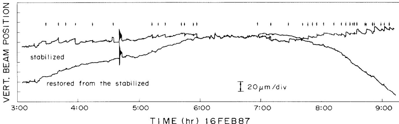
Fig. 6 Suppression effect of the digital feedback system. The upper trace is the stabilized beam position signal and the arrows indicate where a command "up" or "down" was given to the COD correction system. The lower curved trace is restored from the stabilized one. The joggle at 4:40 was due to earthquake.
