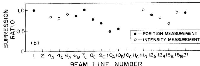
Fig. 4 Suppression ratio of the noise amplitude taken with closed feedback loop to that taken with open loop. Solid circles for beam lines where beam position was measured; open circles for lines where only intensity ratio was measured.
