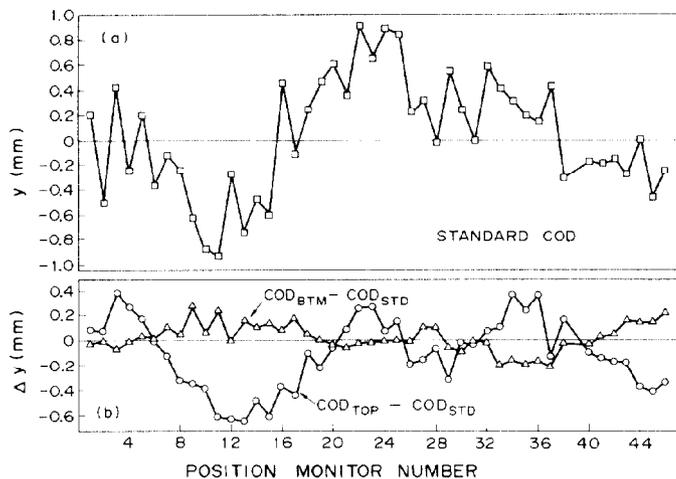
Fig. 5 (a) COD measured at the standard point indicated in Fig. 1. (b) Difference of COD between TOP (BOTTOM) and STANDARD points defined in Fig. 1.
