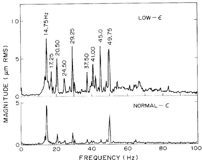
Fig. 2 Beam noise spectra taken at BL 21 with a wire monitor for normal- and low-emittance modes.
