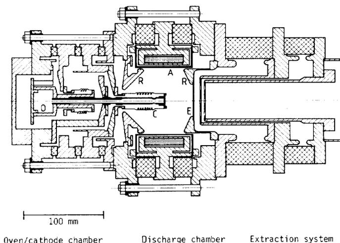
Fig. 1. Hot-running version of CHORDIS with internal oven. O, oven; R, reflector electrode; A, anode; C, cathode; E, extraction system.
