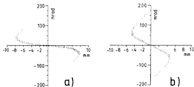
Fig. 3 a and b. Emittance patterns of convergent ion beams, produced by the extraction system according to Fig. 2. Ion species: argon; beam energy: 95 keV. Transported currents: 114.5 mA (case a) and 110 mA (case b).
