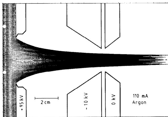
Fig. 2. Large-area, single-aperture extraction system for CHORDIS, producing a convergent beam. Computer simulation by AXCEL-GSI.
