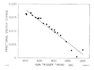
Fig. 3. Observed energy change at the end of Sector 0 as a function of timing changes introduce in the electron gun trigger circuit. The origin is arbitrary for both scales. Relative to the scale shown, the best bunching is at a gun timing of 150 ps. The slope of the linear fit is is  $-2 \times 10^{-5}$  ps<sup>-1</sup>.
