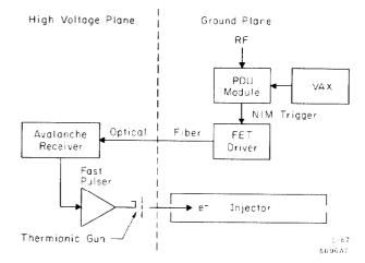
Fig. 2. Schematic diagram of the fiber optic link.
