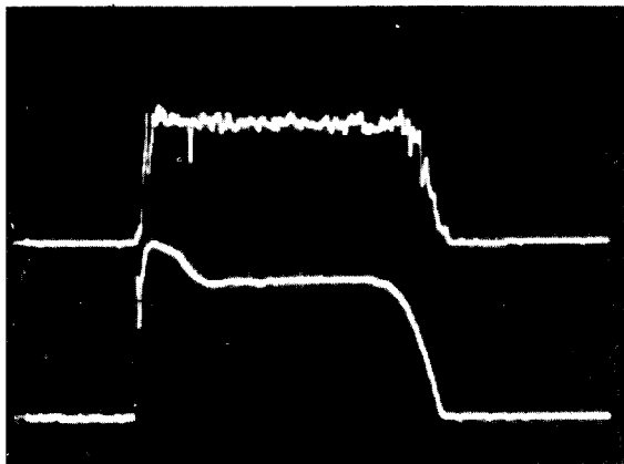
Fig. 4 Oscillogram showing quiescence of the ion beam when the plasma density is optimized to the extractor. Upper trace: beam current, 40 ma/cm. Lower trace: arc current, 50 A/cm. Sweep speed: 50 microseconds/cm.
