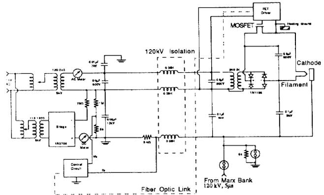
Fig. 2 : Heating and Isolation System
