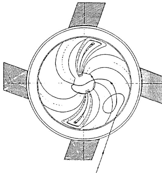
FIG. 7 -- Preliminary design of a separated sector 6 TM SC cyclotron for 400 MeV/A light heavy ions: the EULIMA project.
