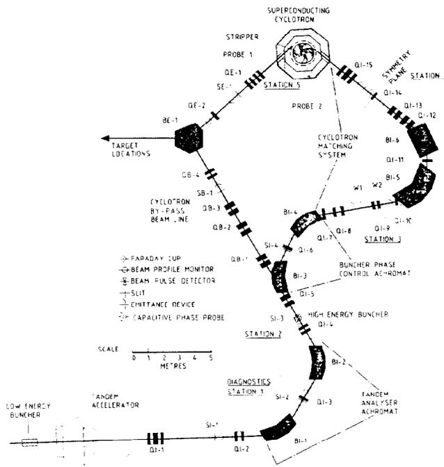
FIG. 1 -- Layout of the Chalk River Tandem Accelerator Superconducting Cyclotron (TASCC) showing the MP-tandem injector, the matching beamline, and the extracted-beam line.
