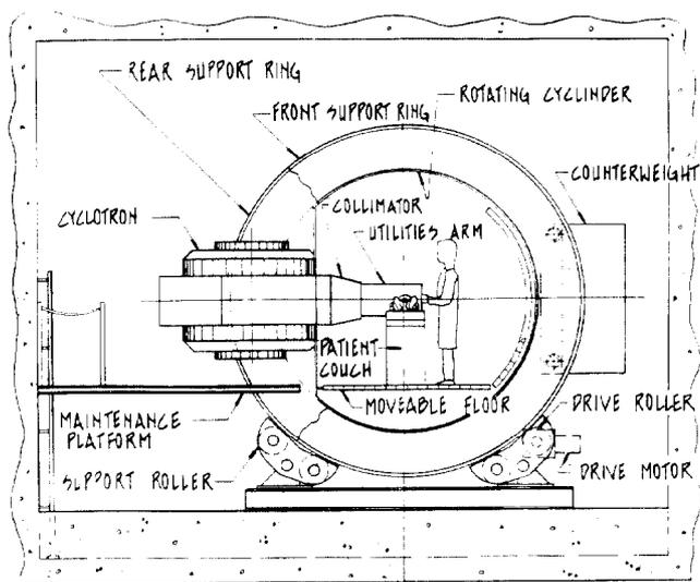
FIG. 2 -- Schematic view of the K100 neutron therapy cyclotron on a gantry to allow variations of the beam direction over a full 360°.
