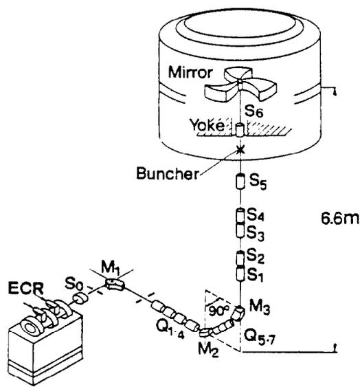
FIG. 5 -- Perspective view of the Milan ECR source and axial injection system into the K800 SC cyclotron.
