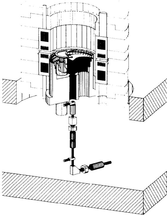
FIG. 6 -- Cutaway view of the AGOR SC cyclotron magnet which has 350 tons of steel and will operate over a dynamic range of 1.75T to 4.07T. It is a 3 sector machine with additional smaller valleys in the center of each hill to permit acceleration of up to 200 MeV protons. The unusual splitting of the 2 pairs of main coils are seen here. The axial-injection system is also shown.
