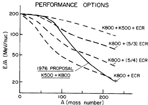
FIG. 4 -- Curves of E/A vs A for several scenarios of K800 cyclotron operation. (5/3)ECR means an ECR with charge state output 5/3 times the charge states achieved by ECR ion sources in 1986.
