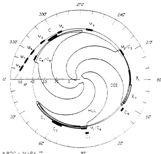
FIG. 3 - Section view of the median plane of the MSU K800 SC cyclotron. For Scale: the outside diameter of the cryostat, the largest circle shown 2.9 m.
