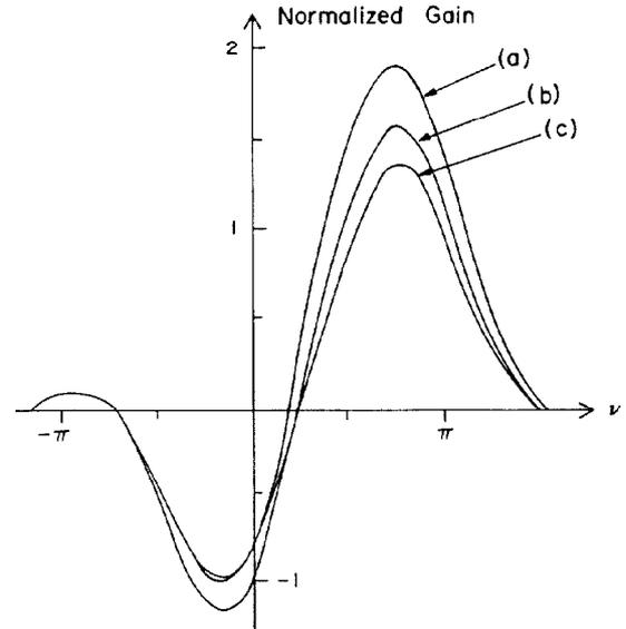
Fig. 5. Normalized gain versus frequency mismatch for  $\lambda = 1.25 \mu\text{m}$  and edge emittance of  $\epsilon_N = 10 \text{ mm mrad}$ . Curves (a), (b) and (c) correspond to results obtained with currents of  $I = 4.0, 2.0$ , and  $0.5 \text{ A}$ , respectively.
