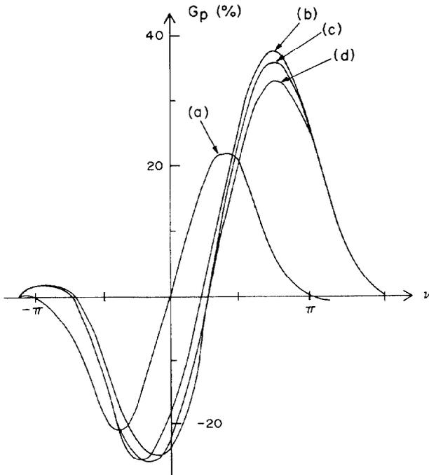
Fig. 4. Power gain,  $G_p$ , versus frequency mismatch,  $\nu$ , at  $\lambda = 1.25 \mu\text{m}$  with  $\gamma_o = 150$ . Curve (a) is based on 1-D gain formula. Curves (b), (c) and (d) are obtained from simulations with normalized transverse edge emittances of  $\epsilon_N = 5, 10$  and  $20 \text{ mm mrad}$ , respectively.
