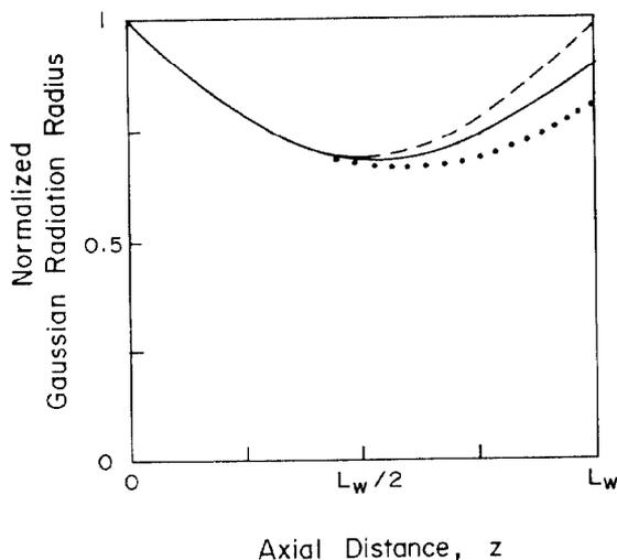
Fig. 6. Normalized  $1/c$  Gaussian radiation field amplitude radius as a function of distance  $z$  in the wiggler with  $\lambda = 1.25 \mu\text{m}$  and edge emittance  $\epsilon_N = 10 \text{ mm mrad}$  for three different currents: (---)  $I = 0.5 \text{ A}$ , (—)  $I = 2 \text{ A}$  and (.....)  $I = 4 \text{ A}$ .
