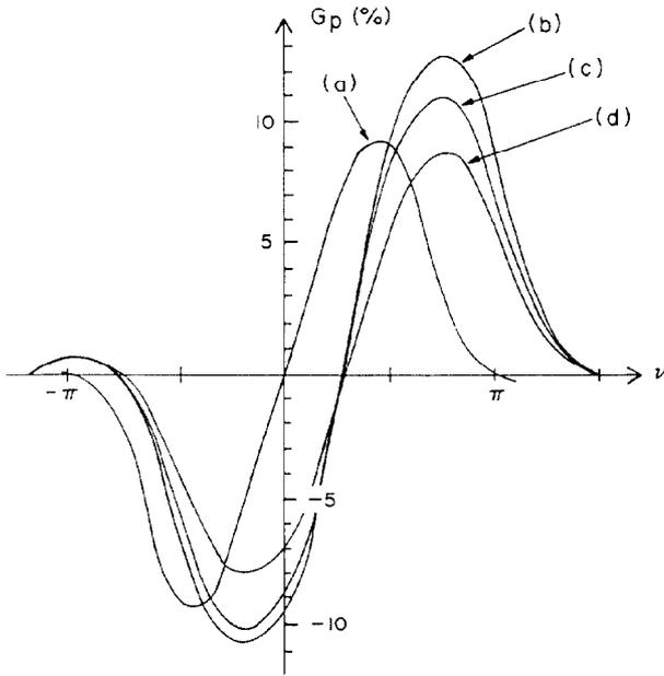
Fig. 3. Power gain,  $G_p$ , versus frequency mismatch,  $\nu$ , at  $\lambda = 0.23 \mu\text{m}$  with  $\gamma_o = 350$ . Curve (a) is based on 1-D gain formula. Curves (b), (c) and (d) are obtained from simulations with normalized transverse edge emittances of  $\epsilon_N = 5, 10$  and  $20 \text{ mm mrad}$ , respectively.
