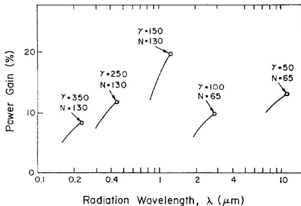
Fig. 2. Small signal power gain versus wavelength based on 1-D calculation.
