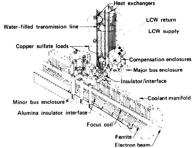
Fig. 5. Ten-cell induction accelerator module on ARC.
