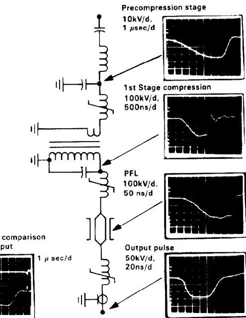
Fig. 3. MAG-I-D voltage waveforms.
