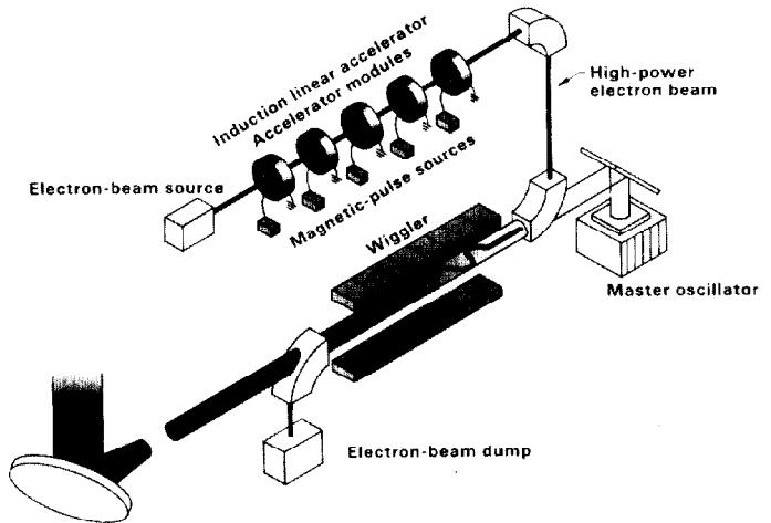
Fig. 1. Component technologies for induction linac FEL amplifiers.
