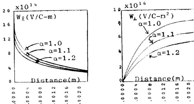
Figure 1: Delta function wake fields at 7.79 GHz, for  $\alpha = 1.0, 1.1, 1.2$ .
