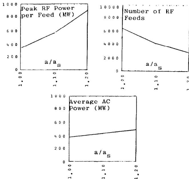
Figure 3: Number of rf feeds per linac, peak rf power per feed, and average ac power per linac versus  $\alpha$ .
