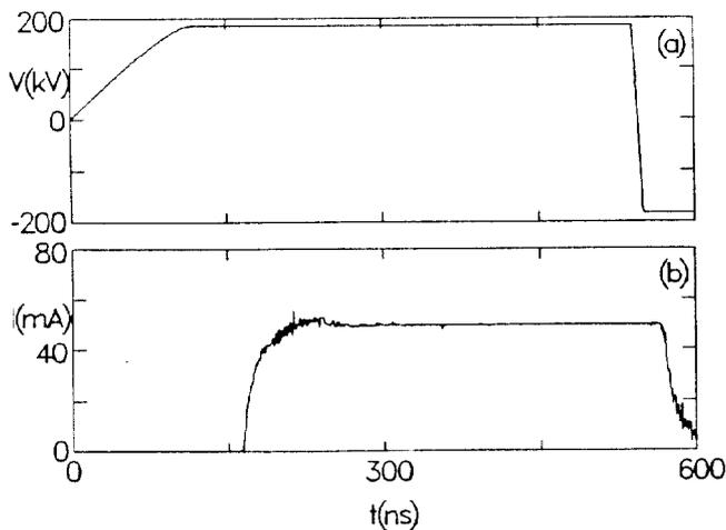
Fig. 3 ISIS simulation showing (a) tailored voltage profile (b) nearly step-function resulting current profile.
