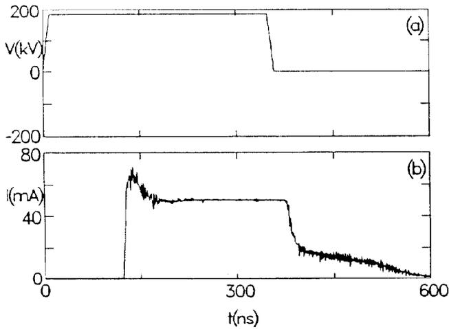
Fig. 2 (a) Voltage profile for 10 ns risetime in ISIS simulation. (b) Resulting current profile showing overshoot.
