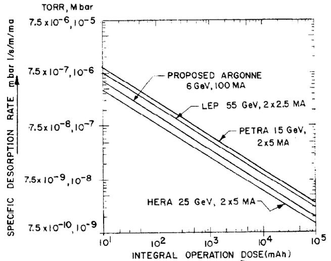
Figure 1 Specific Desorption Rates
