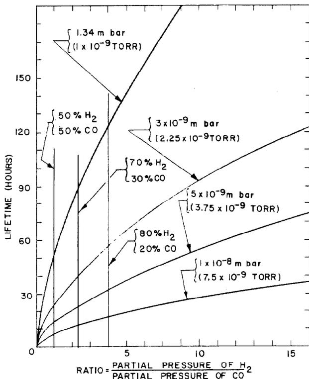
Figure 7 Beam Lifetimes for  $\text{CO}$  and  $\text{H}_2$
