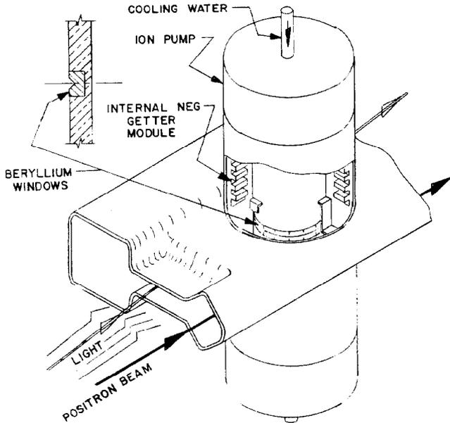
Figure 3 Crotch Absorber Lumped NeG Pumping
