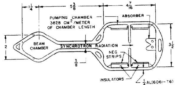
Figure 2 Vacuum Chamber
