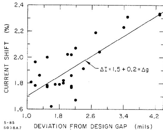
Fig. 6. The correlation between the gap deviation ( $\Delta g$ ) and current adjustment ( $\Delta I$ ).
