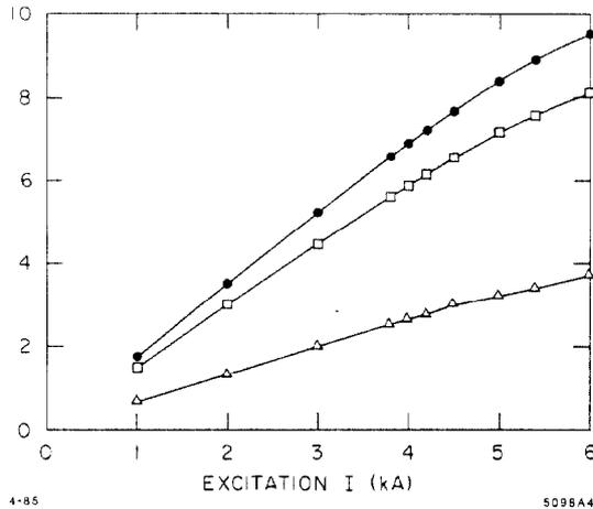
Fig. 4. The dipole ( $\square$ , KG), quadrupole ( $\bullet$ , KG/cm) and sextupole strength ( $\triangle$ , KG/cm/cm) vs.  $I$ .
