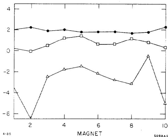
Fig. 5. The center line shift ( $\triangle$ , mil), current adjustment ( $\bullet$ , %), and sextupole deviations ( $\square$ , %) for ten magnets.
