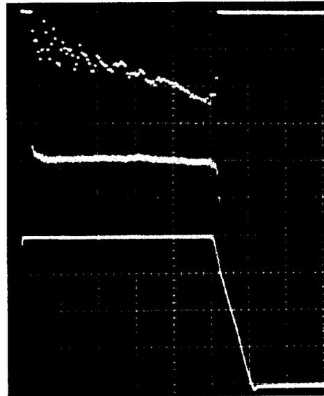
Fig. 6. Final pulse shape with applied function generator. The 100-point function applied is shown at the top at 2 V/division. The lower trace is the final pulse (200 μs/division, 500 A/division), and the middle trace is an expanded view of the flat top at 5 A/division.
