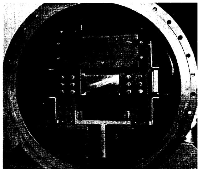
Fig. 1. Kicker magnet unit in vacuum chamber.
