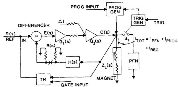
Fig. 3. Active feedback regulator functional diagram.
