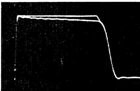
Fig. 5. Switchyard kicker PFN current with (upper trace) and without feedback applied (200μs/division, 500 A/division).
