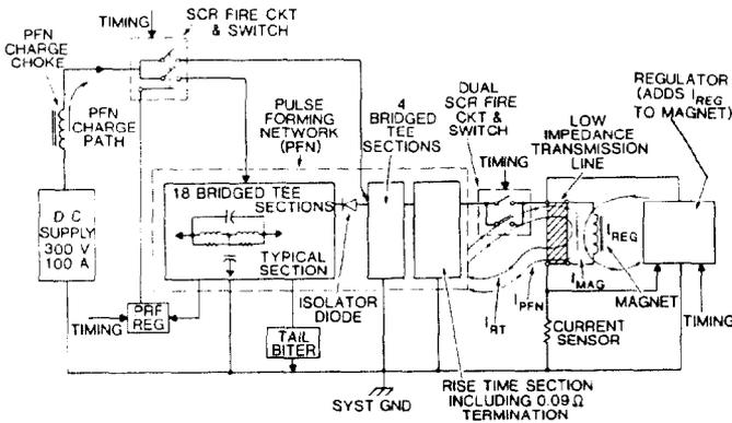
Fig. 2. Functional diagram of the modulator, showing three current loops through the magnet.
