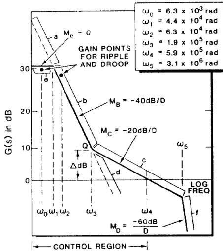
Fig. 4. Bode diagram for the regulator. Abscissa (frequency) is not to scale.
